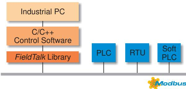
Typical applications are Modbus based Supervisory Control and Data Acquisition Systems (SCADA), Modbus data concentrators, Modbus gateways, User Interfaces and Factory Information Systems (FIS).
