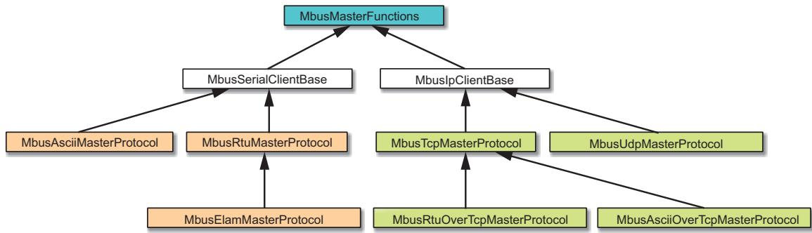
The base class **MbusMasterFunctions** contains all protocol unspecific functions, in particular the data and control functions defined by Modbus. All Modbus protocol flavours inherit from this base class.
