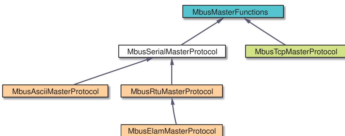
The base class **MbusMasterFunctions** contains all protocol unspecific functions, in particular the data and control functions defined by Modbus. All Modbus protocol flavours inherit from this base class.
